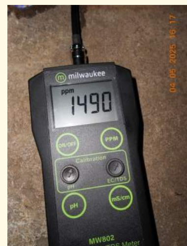
After turning the calibration adjustment knob, the readout is 1490 and TDS calibration is complete
