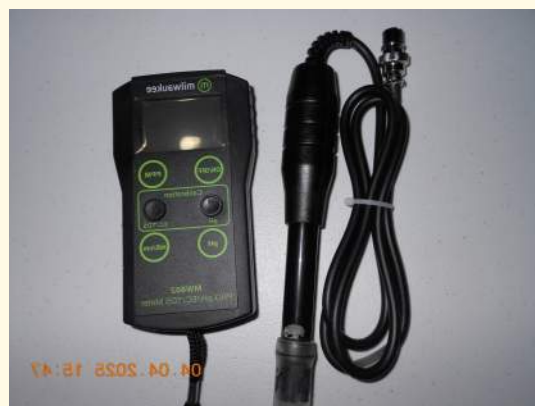
Closeup of the Milwaukee Instruments MW802 PRO pH/TDS/EC meter and probe
