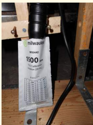
Probe Immersed in a pouch of TDS calibration fluid
